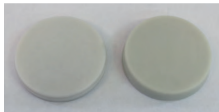
SILBOND 006 MST in PMMA (links) und in UP-Harz (rechts) SILBOND 006 MST in PMMA (left) and in UP resin (right)
